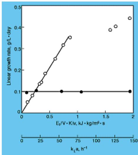
**Figure (10) : The effects of the light supply coefficient ( $E_t/V \cdot K_{iv}$ ; ) and the volumetric oxygen transfer coefficient ( $k_{La}$ ; ) on the photoautotrophic linear growth rate of *C. pyrenoidosa*.**
