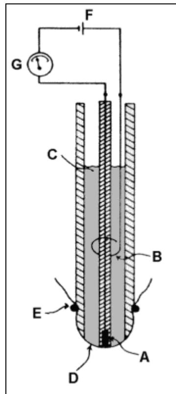
**Figure(3):**The Clark-type electrode consists of a Pt- (A) and a reference Ag/AgCl-electrode (B) covered by a film of half-saturated KCl electrolyte (C) enclosed within a Teflon membrane (D) which is held in place by a rubber ring (E). Originally developed for measuring oxygen gas, it is only a matter of polarity, whether the electrode senses hydrogen or oxygen gas. For hydrogen measurements 600 mV (F) are supplied, and the electrodes output (G).
