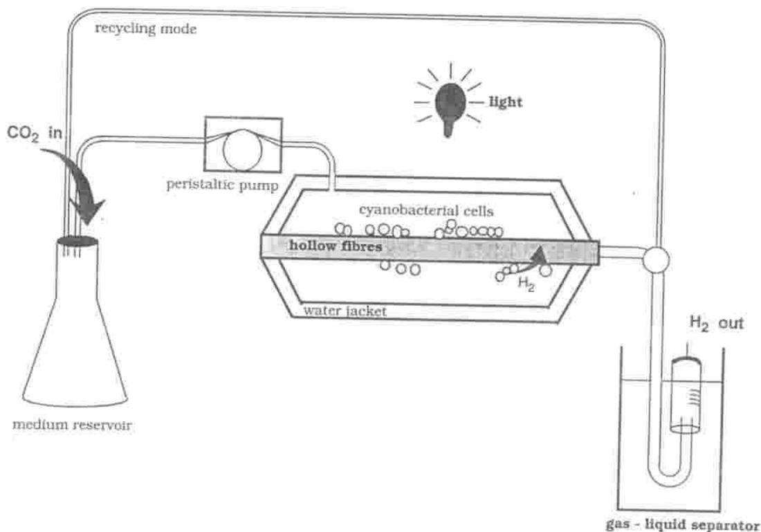
Figure (7): Schematic diagram of hollow fibre photobioreactor for continuous production of hydrogen by immobilized cyanobacteria.
