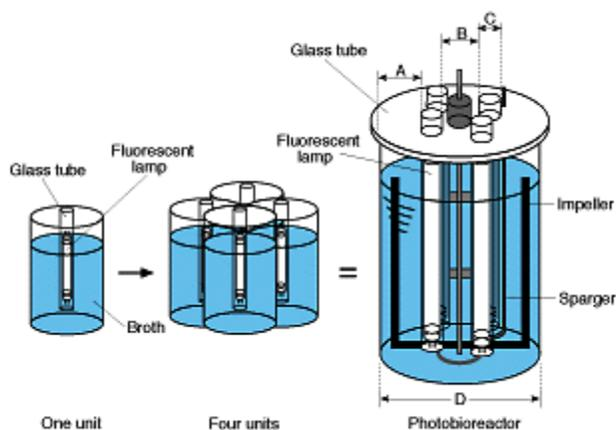
**Figure (12): The novel photobioreactor. A: The distance from the reactor wall to the glass tube (2.3 cm). B: The distance between the opposite glass tubes (4.6 cm). C: The diameter of the glass tube housing the fluorescent lamp (2.4 cm). D: The diameter of the reactor (14 cm). Source: Adapted from Reference 21.**
