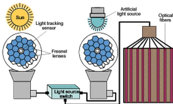
Figure (15): System used for light collection and distribution through the optical fibers. An artificial light source supplements solar energy during the night or on cloudy days.
