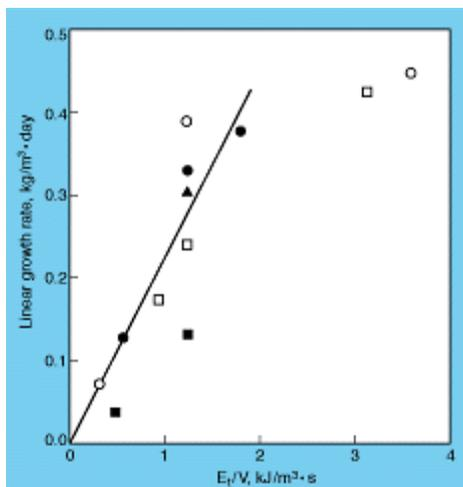
**Figure (8): The effects of light energy supplied per unit volume of photobioreactor ( $E_t/V$ ) on the linear growth rates of *Chlorella pyrenoidosa* in cuboidal photobioreactors. The depths of the photobioreactors were 0.02 m, 0.04 m, 0.06 m, 0.08 m, and 0.16 m.**
