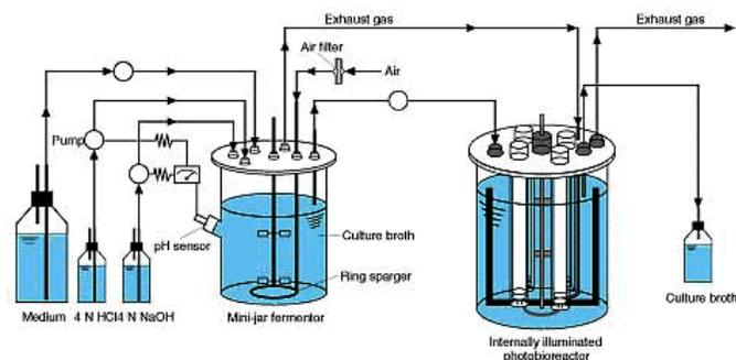
**Figure (13): System used for the continuous sequential heterotrophic-photoautotrophic cultivation of *C. pyrenoidosa*. The working volumes of the mini-jar and the photobioreactors were 2.0 and 3.0 L, respectively.**
