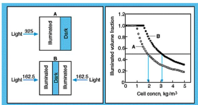
**Figure (9): The effects of cell concentration on the illuminated volume fraction of a cuboidal photobioreactor illuminated from one surface (A) or from two surfaces (B). Although the light energy supplied per unit volume (in  $\mu\text{mol}/\text{m}^2\text{s}$ ) is the same in the two photobioreactors, the calculated light distribution coefficients were  $1.9 \text{ kg}/\text{m}^3$  and  $3.1 \text{ kg}/\text{m}^3$  for photobioreactors A and B, respectively.**
