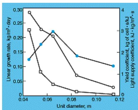
**Figure (11):** The effects of unit diameter on linear growth rate, yield coefficient, and light supply coefficient of *C. pyrenoidosa*. Each unit was internally illuminated by a 4-W fluorescent lamp producing a light intensity of 163  $\mu\text{mol}/\text{m}^2\text{s}$ .
